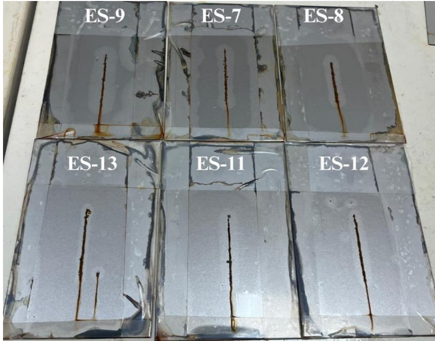
Figure 12. Appearances after 100 hours of corrosion testing
