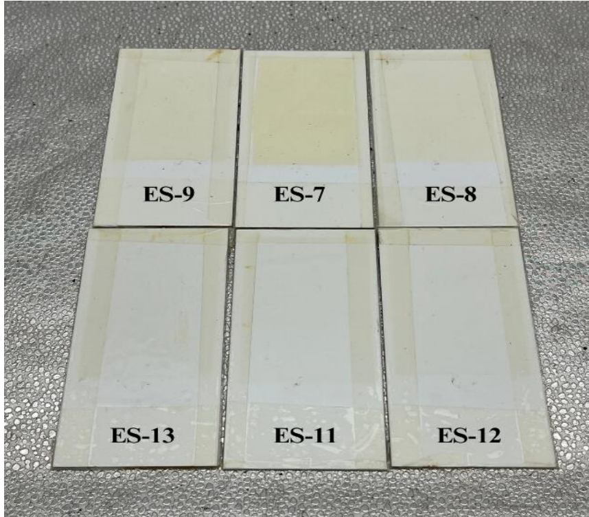
Figure 11. Appearances after 100 hours of UV testing
