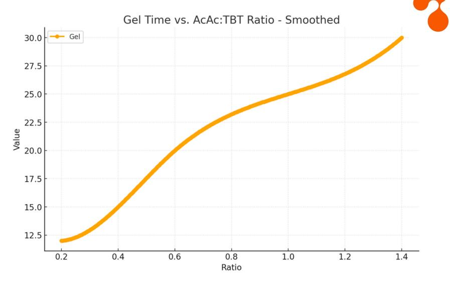
Impact resistance is increasing with an increase in TBT treatment content of the catalyst. The gelation time increased with the increase in the TBT treatment ratio. TBT: AcAc ratio optimised at 1: 0.8 ratio
