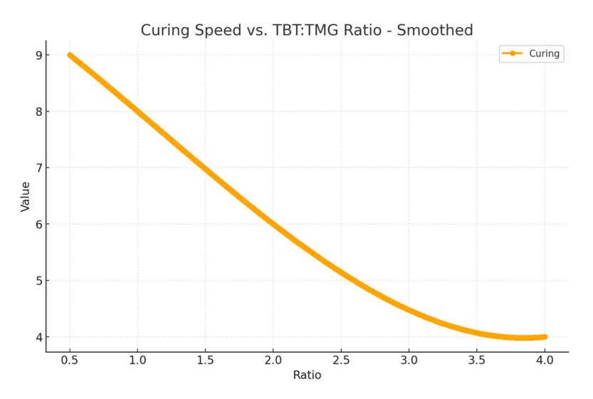
Adhesion increases with an increase in TBT content up to 3 times that of TMG in the catalyst mixture. Curing speed properties accelerate with the increase in the TMG ratio. TBT: TMG ratio optimised at 1: 0.75 ratio.
