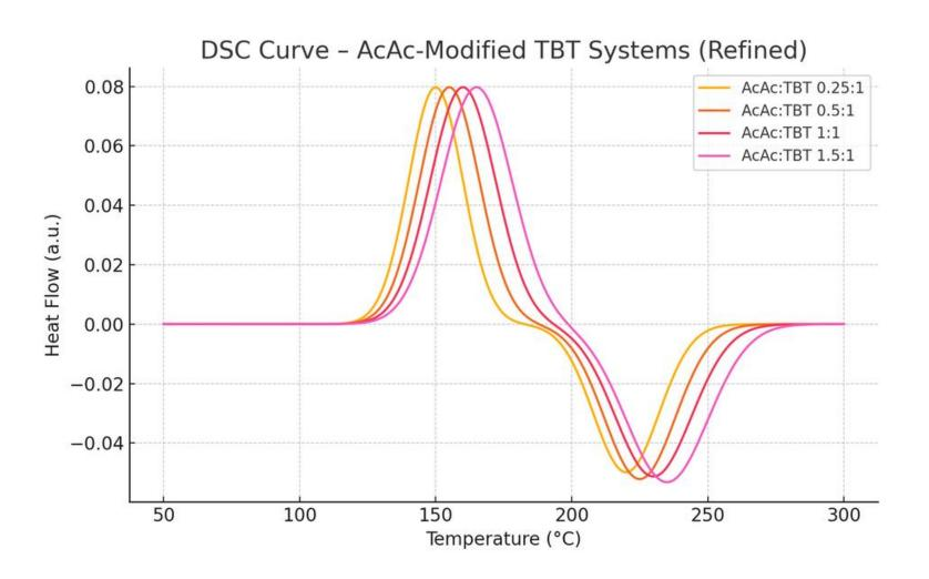
The Tg temperature differs specifically from the catalyst ratio. The change in the catalyst ratio changes the Tg of the dry film. Same thing same in the weight loss with temperature increment.
