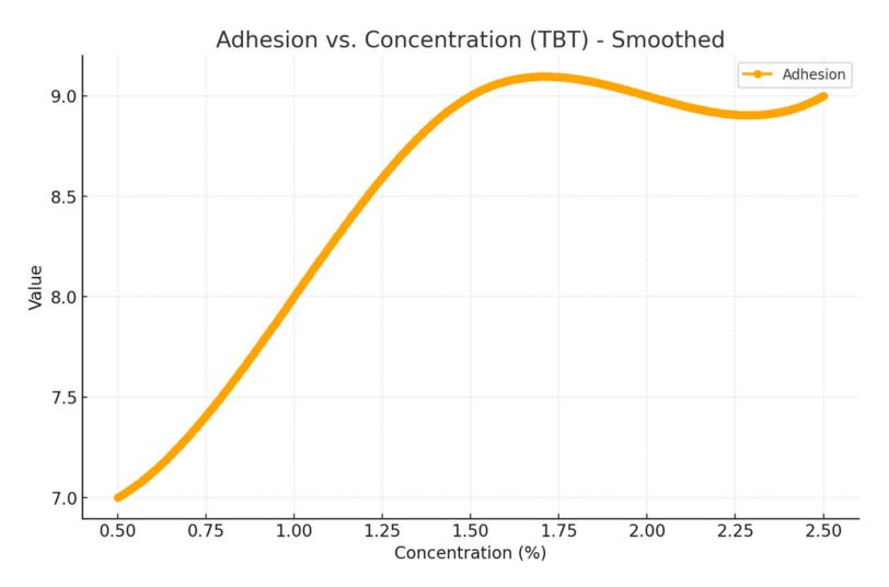
Adhesion requires TBT curing for ambient curable silicone resins. Increase in the concentration helpsadhesion but cross-linking degree increament causes loss in adhesion.
