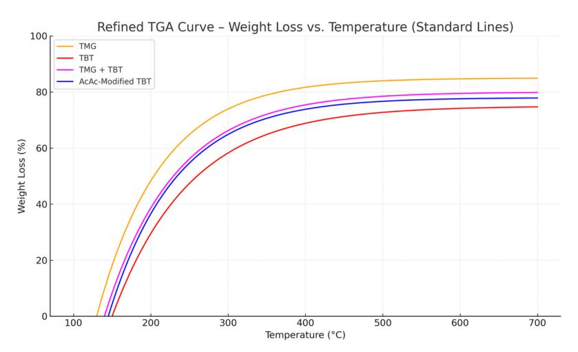
The Tg temperature differs specifically from the catalyst type. The change in the catalyst type changes the Tg of the dry film. Same thing same in the weight loss with temperature increment.
