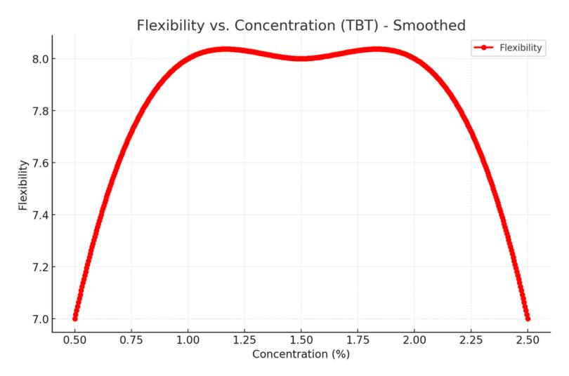
Flexibility is increasing up to 2% of the catalyst concentration. Higher dosages make the film more brittle. TMG increases the brittleness compared to the TBT.
