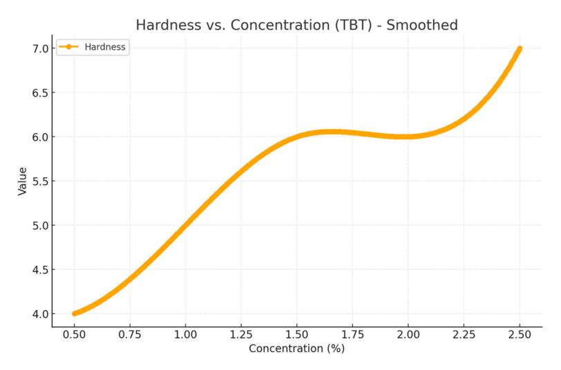
TMG improves the hardness of the film. Surface curing is very affected by curing with TMG. TBT can also increase hardness but requires high catalyst dosages.
