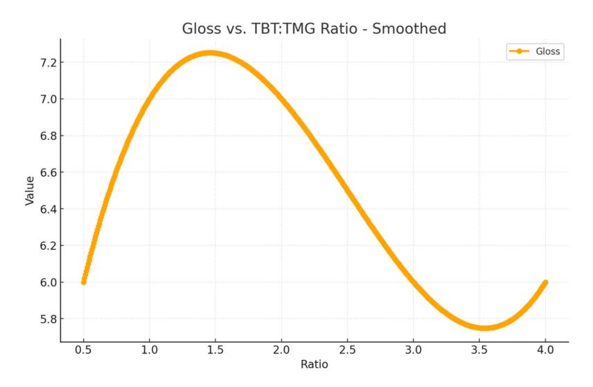
Impact resistance is increasing with an increase in TBT content of the catalyst mixture. The gloss properties decrease with the increase in the TBT ratio. TBT: TMG ratio optimised at 1: 0.5 ratio
