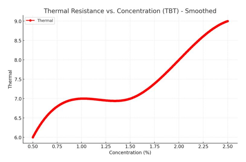
Thermal resistance increased with the TBT catalyst. TMG does not react with resins; however, TBT reacts with the resin and creates Ti-O-Si units which helps thermal stability.
