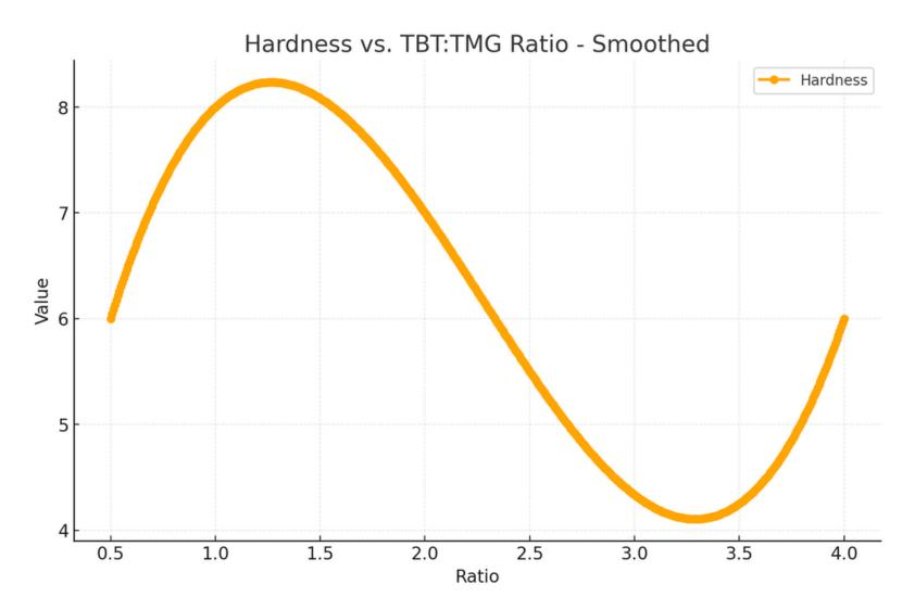
Flexibility is decreasing with an increase in TMG content of the catalyst mixture. Hardness properties vary with the change in the TMG ratio. TBT: TMG ratio optimised at 1: 0.75 ratio.
