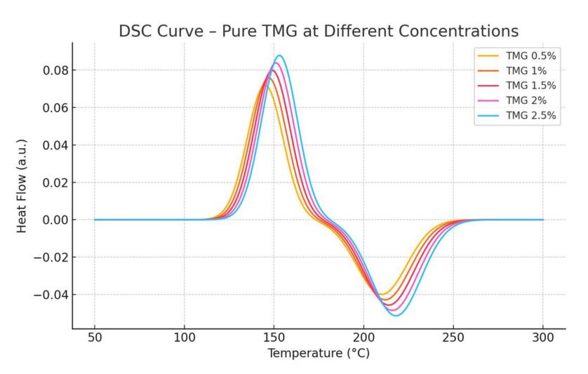
The Tg temperature differs from both the concentration and the catalyst type. An increase in concentration increases the Tg of the dry film. High concentration of the catalyst causes an increase in cross-linking at higher temperatures.
