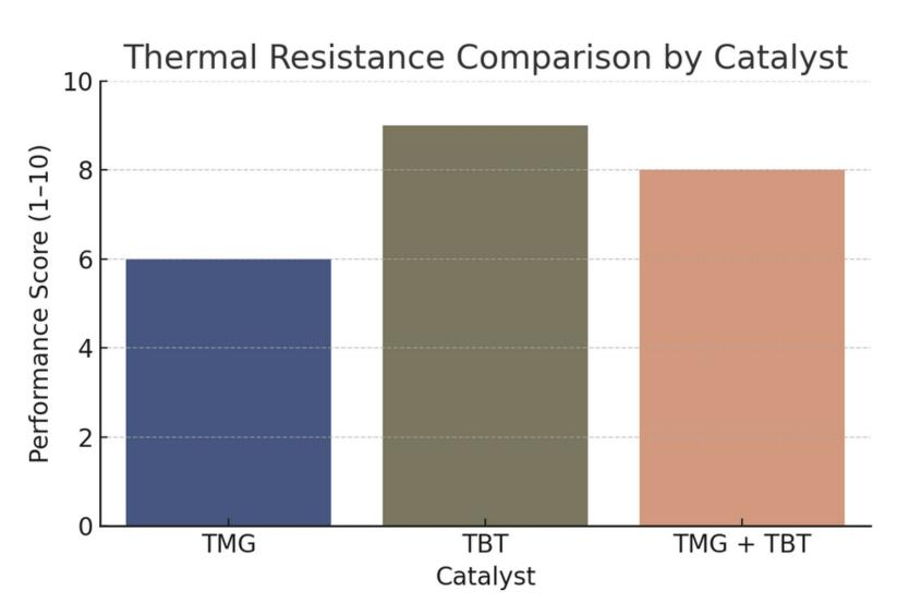
Hardness also increased with TMG, but TMG usage decreases thermal stability. The best option to have both thermal resistance and good hardness with low catalyst usage requires mixing of catalysts.
