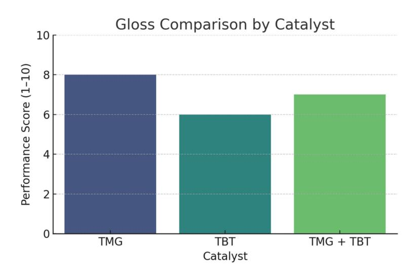
Methyl-phenyl modified silicone resins should be cured with the catalyst mixture because of their highly non-polar structure. To have good results with only TBT requires the high amount of catalyst dosages.
