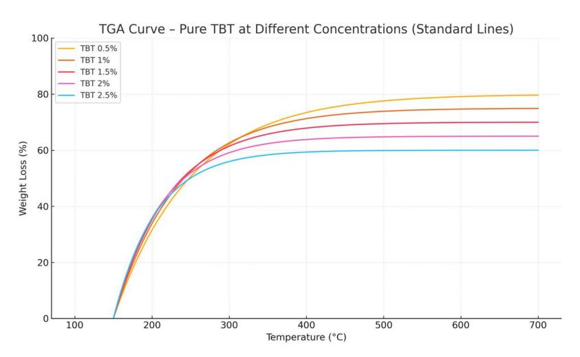
With higher dosages, the cross-linking degree is higher, which gives lower weight loss in TGA analysis. TBT improves thermal stability. Degradation starts at higher temperatures with TBT curing.
